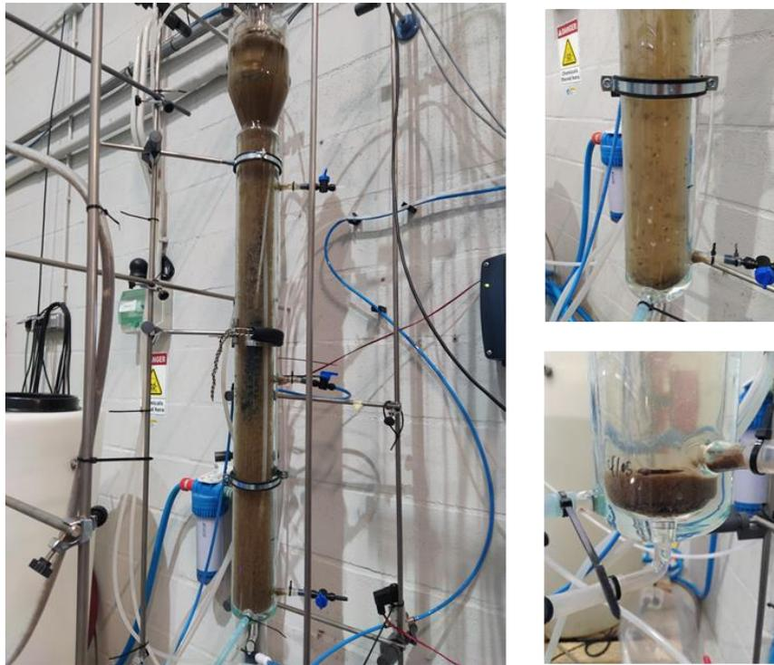
Figure 15. Partial nitritation reactor experimental set-up
