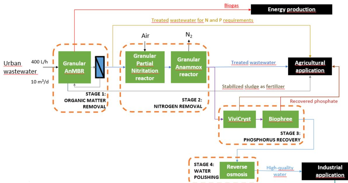
Figure 11. Treatment process diagram for CS5
