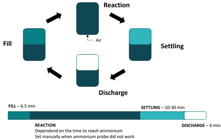
Figure 16. Sequential batch reactor operation (SBR) set-up. Consisting of a filling phase of 6.5 minutes, a reaction phase, settling phase that was decreased during the operational phase to achieve fast settling biomass, and finally a discharge phase.
