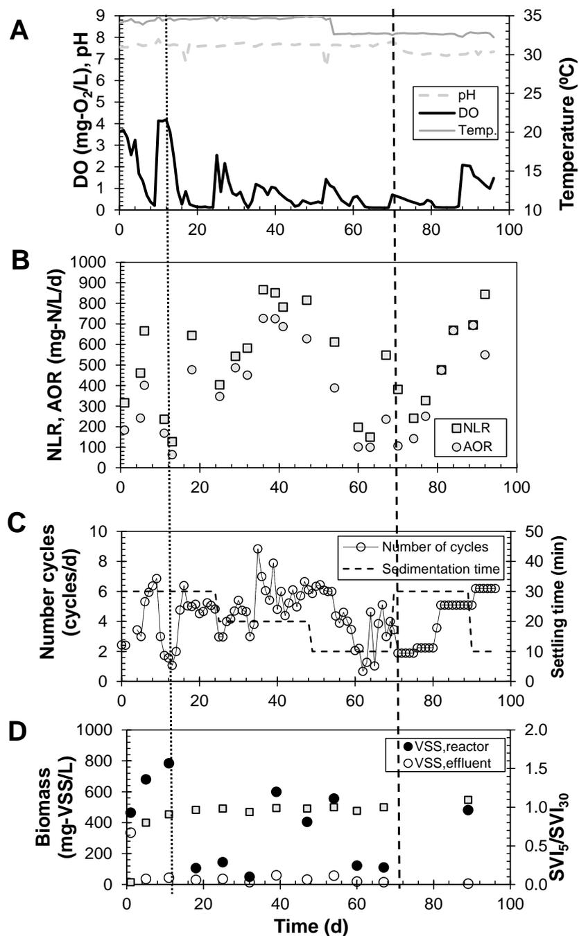
Figure 17. Partial nitrification reactor operation data. A) pH, dissolved oxygen (DO) and Temperature, B) Nitrogen loading rate (NLR) and ammonium oxidation rate (AOR), C) Number of cycles and sedimentation time, D) Biomass and SVI.. First dotted line indicates a technical problem with the discharge valve. The second dashed line indicates a reinoculation and a switch to cycle length control instead of ammonium concentration-based control.
