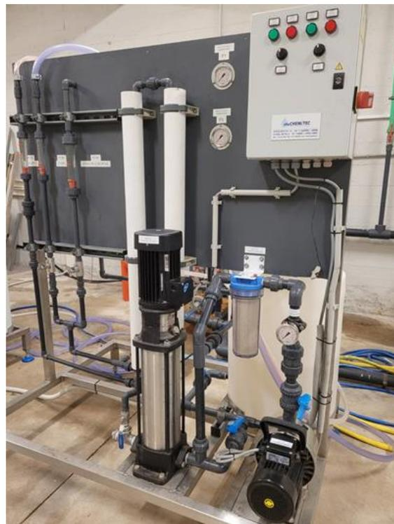
*Figure 3. RO unit for bench scale tests*
