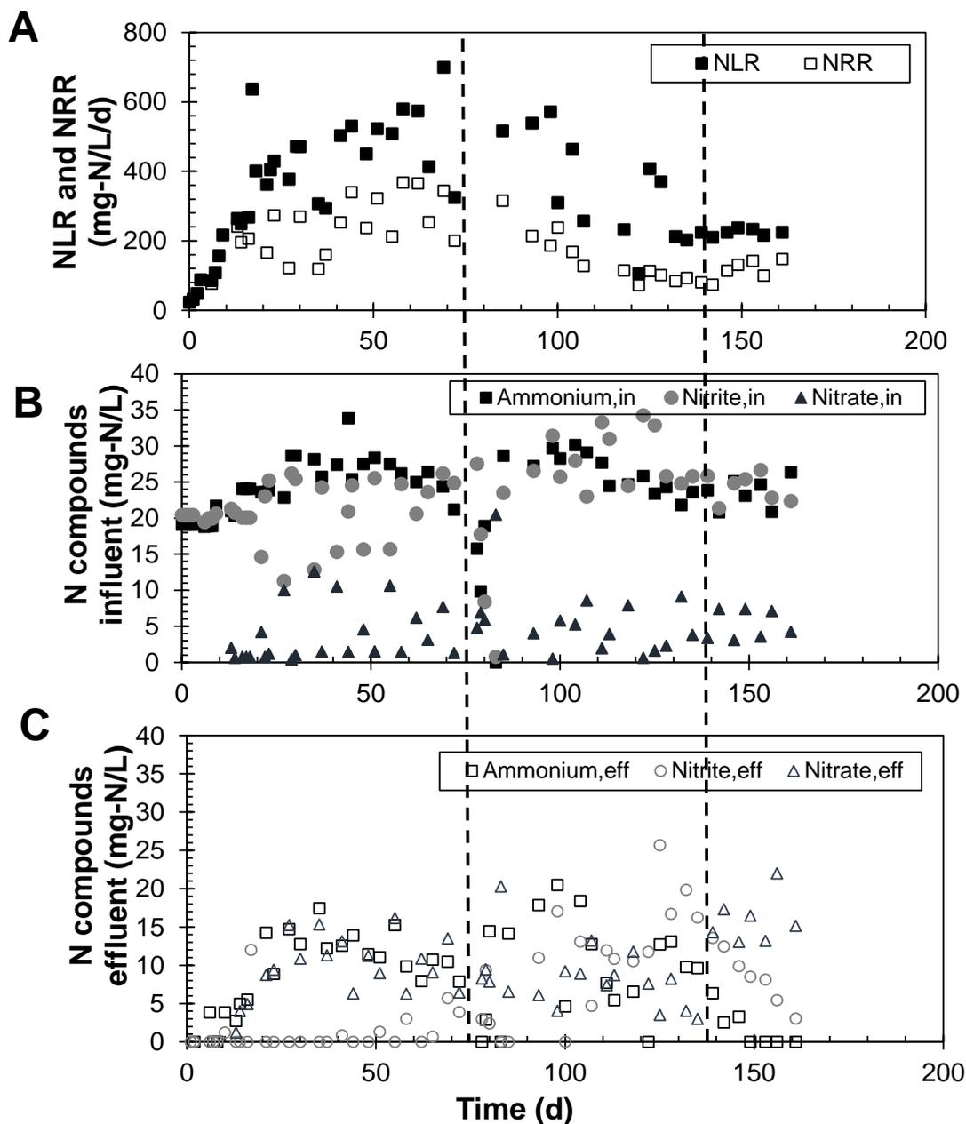
Figure 19. Anammox reactor operation data. First dashed line indicates when air entered the reactor due to a technical issue. Second dashed line indicates recirculation implementation. A) Nitrogen loading rate (NLR) and nitrogen removal rate (NRR). B) Nitrogen compounds concentration in the influent tank, C) Nitrogen compounds concentration in the effluent.
