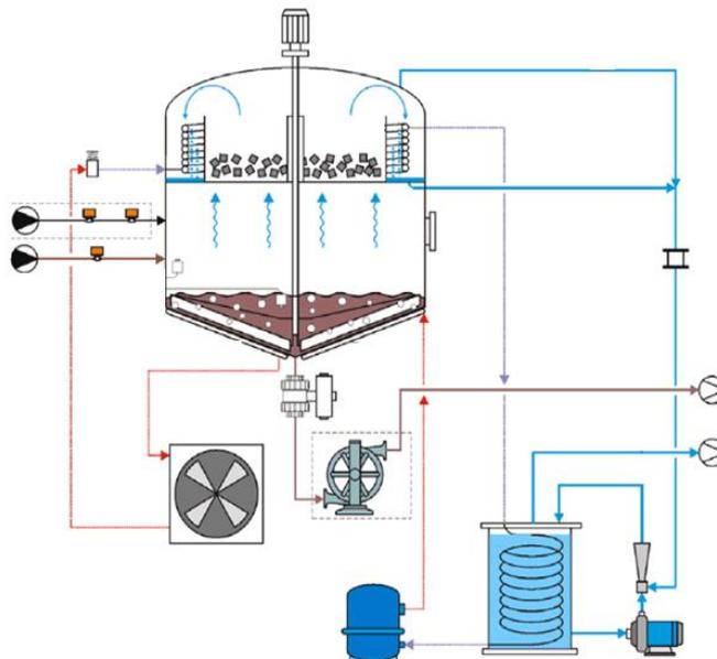
Figure 9. Working scheme of crystallizer.
