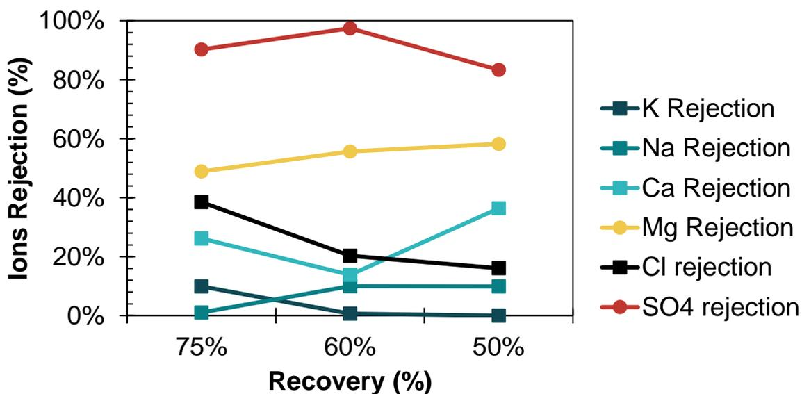
Figure 7. Ions rejection for 50%, 60% and 75% recovery (pH=6) without recirculation flow
