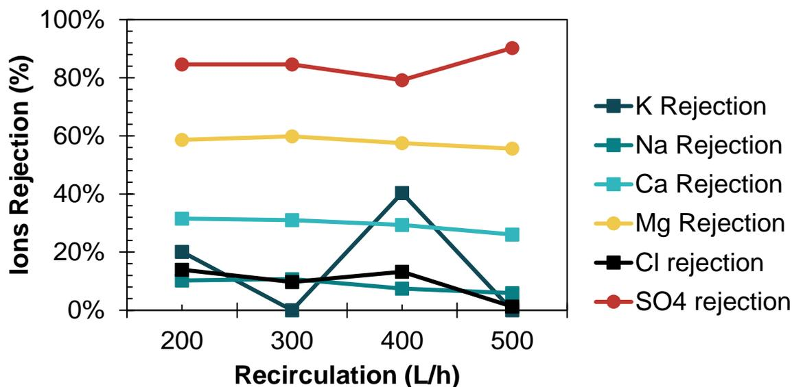
Figure 4. Ions rejection for 75% recovery (pH=7.3) at different recirculation flows
