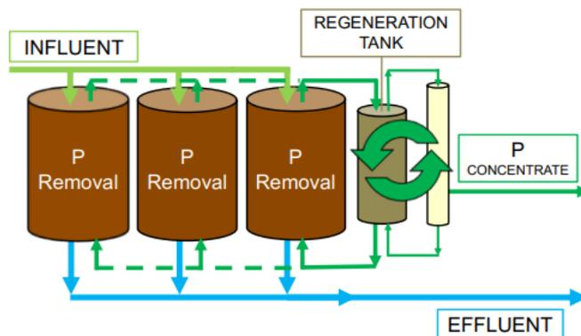
Figure 25. Simplified process scheme of the BioPhree adsorption system (pre-treatment (filtration) not shown)
