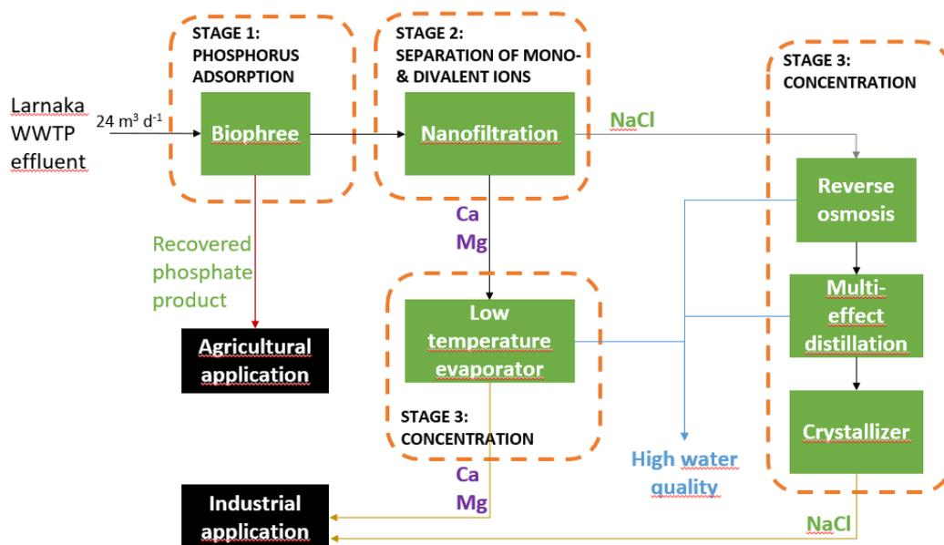
Figure 1. Treatment process diagram for CS4
