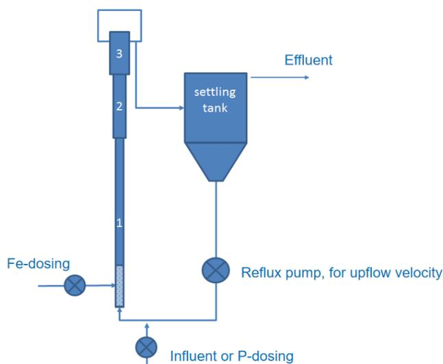
Figure 20. Diagram of the bench-scale crystallizer
