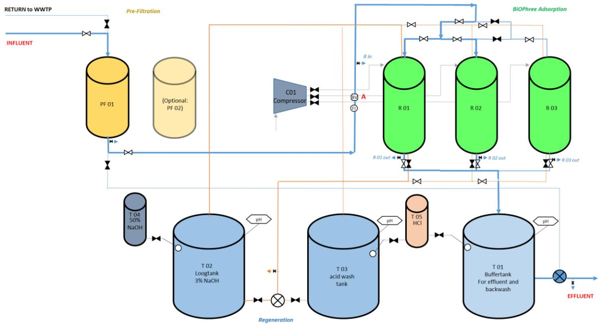
Figure 26. Process flow diagram of the BioPhree pilot
