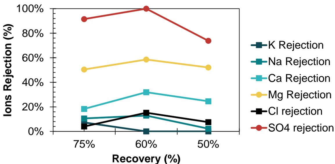
Figure 6. Ions rejection for 50%, 60% and 75% recovery (pH=7.3) without recirculation flow
