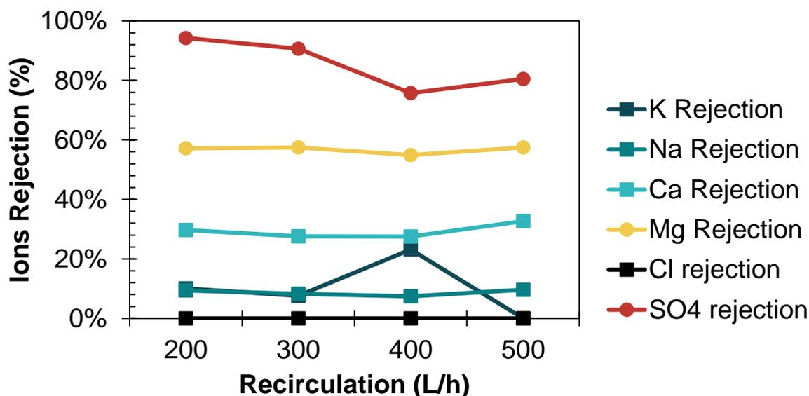
Figure 5. Ions rejection for 60% recovery (pH=7.3) at different recirculation flows
