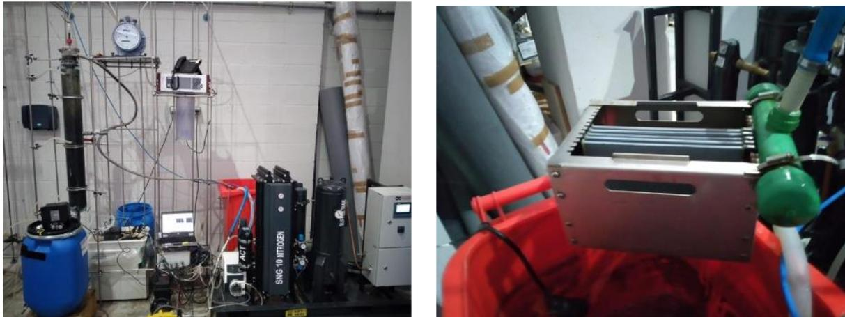
*Figure 13. Anaerobic membrane bioreactor experimental set-up*
