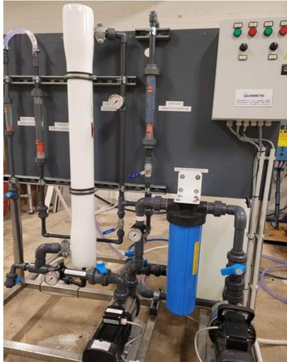
*Figure 2. NF unit for bench scale tests*
