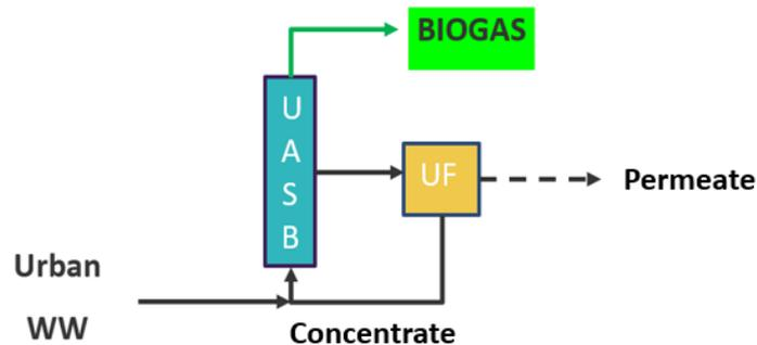
Figure 12. Diagram of the configuration of the granular anaerobic digestion membrane (AnMBR) using a Upflow Anaerobic Sludge Blanket (UASB) reactor
