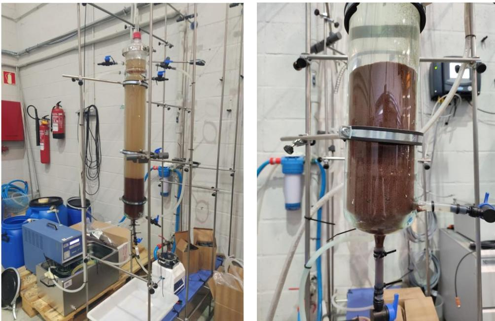
Figure 18. Anammox UASB reactor experimental set-up
