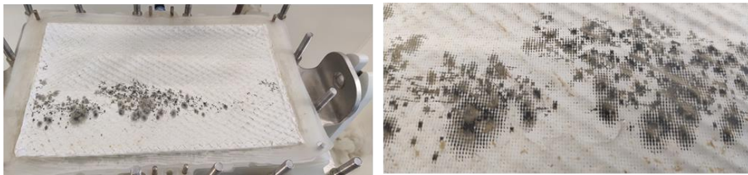
Figure 18. ePTFE membrane's surface after the MD test.
