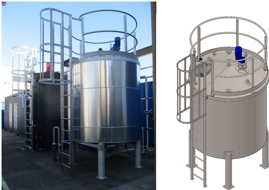
Figure 5: The reactor tank for alkalisation and heating up the excess sludge.
