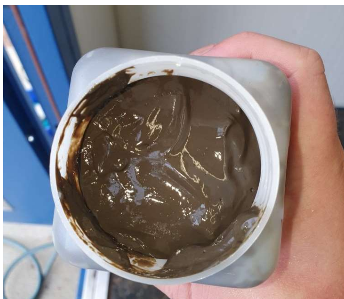
Figure 17: Kaumera extracted from excess sewage sludge from the MWWTP Faro Olhão.
