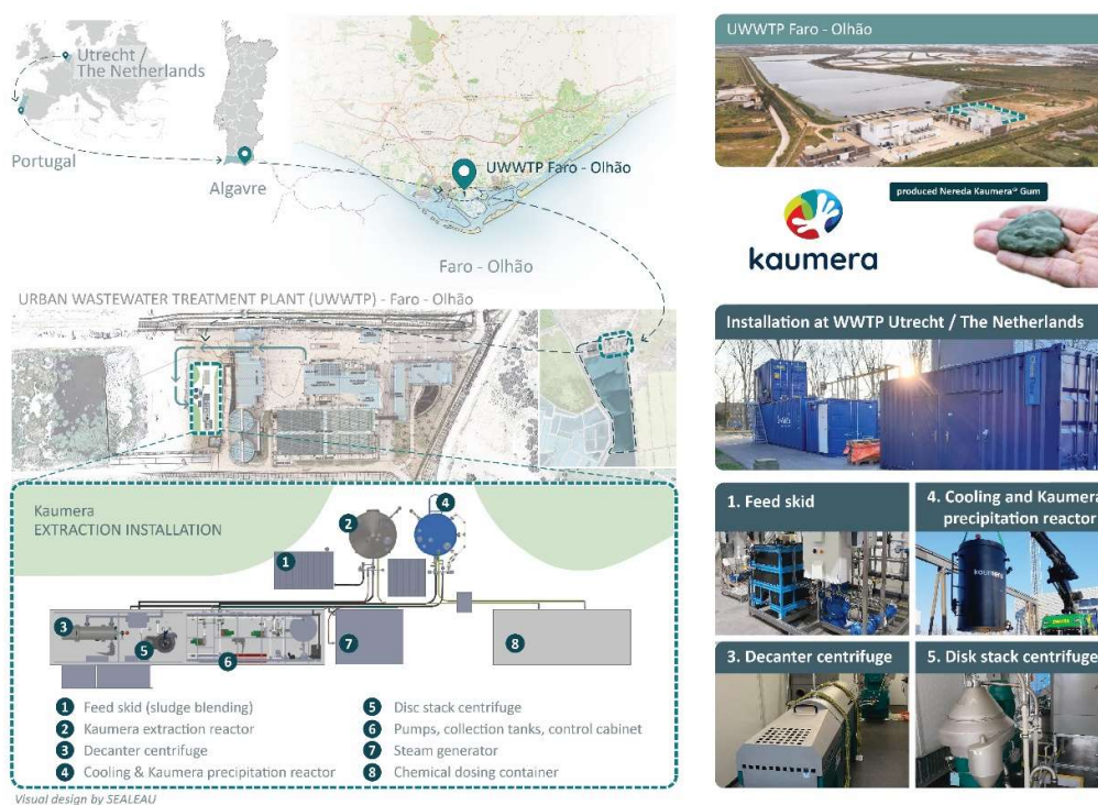
Figure 12: Overview on the main CS3 equipment and the location of CS3 in Faro, Portugal
