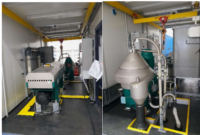
Figure 10: Decanter centrifuge (left) and disc centrifuge –a.k.a. separator (right).
