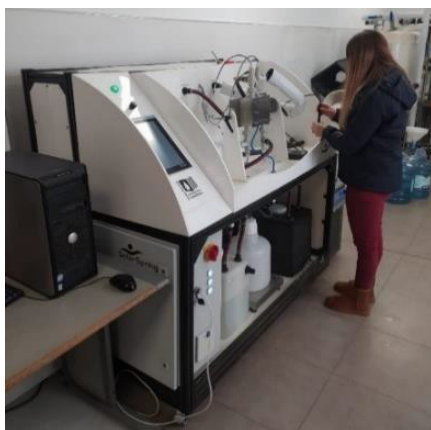
Figure 17. Pilot plant to test membrane distillation materials and applications
